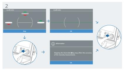
**Note:** The short horizontal white line inside the circle is moving vertically and it represents the rotation around the Y-axis. When it matches the white line, the device will be in balance with the Y-axis, then the line color will turn from white to green.
